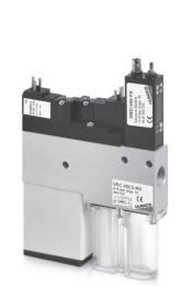
Vacuum generators with integrated suction and blow-off valves, as well as a monitoring system (vacuum switch). Series VEC compact ejectors allow to control suction and blow-off individually without using external valves.
