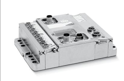
The serial module CX2 can be used both integrated on different valve series (Series 3, Series H) and as external component. This device allows the connection of up to a max of 64 solenoids and 64 inputs on the base unit, so applications other than pneumatics are a possibility. Thanks to its aluminium support structure, this solution is IP65 rated with high mechanical strength. It is therefore suitable for mounting in arduous conditions.
