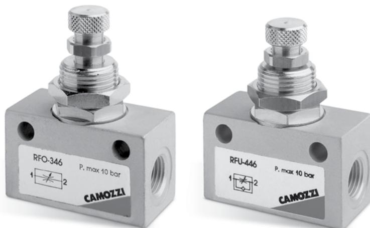
The unidirectional flow controllers are equipped with M5, G1/8 and G1/4 ports, each of which is available with two different types of adjustment (see diagrams), except for the M5. They are used mainly for controlling the speed of cylinders. They may be mounted on control panels or cylinders, as required.
