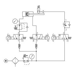
For a correct use of the rod lock Mod. RLC a pneumatic connection is recommended (as shown in the examples).
