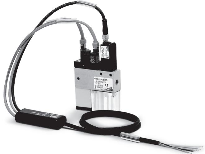
The air saving circuit, when used, switches the suction signal to "ON" apart from the fact that the ejector is NC or NO; this means that, in order to switch the internal loop back to "OFF", it is necessary to activate the signal on the coil controlling it (green cable).
