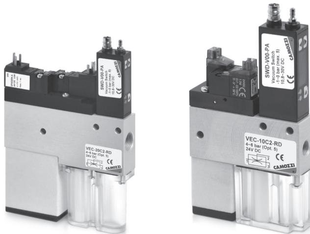
Vacuum generators with integrated suction and blow-off valves, as well as a monitoring system (vacuum switch). Series VEC compact ejectors allow to control suction and blow-off individually without using external valves.
