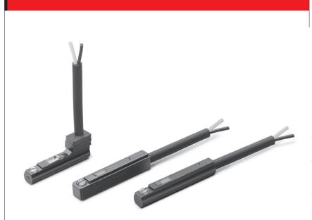
Series CSB/CSC magnetic proximity switches define the position of the magnetic piston. When the internal contact is actuated by a magnetic field, the sensors complete an electrical circuit and provide an output signal to actuate directly a solenoid valve or a PLC.
