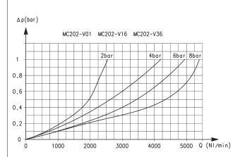
Flow diagram for models: MC202-V01 MC202-V16 MC202-V36
