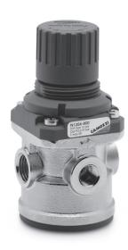
Series N pressure regulators are available with G1/4 and G1/8 ports. Their design incorporates a self relieving diaphragm so as to allow decremental adjustments.
