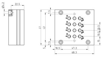
Note: the manifolds are supplied complete with the seals and the valves, fixing screws.
