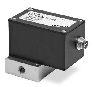
LRPA4 proportional servo valves are valves for the high precision pressure control with integrated closed loop circuit. This is a 3/3-way valve, based on a patented rotating spool system with electronic control of the position, a pressure sensor and an electronic PID-control board.
