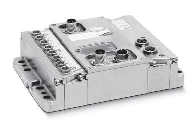
This is a Fieldbus Module with class of protection IP65. Thanks to the high mechanical strength of its Aluminium support structure, it is suitable for mounting in arduous conditions. It can be coupled with electrical input/outlet modules and is able to handle up to a max of 64 solenoids and 64 inputs. Through pre-packaged connection cables, it can be interfaced with multipole valve islands.
