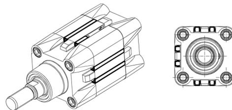
Slot cover profile for cylinders Series: 31 - 31 tandem and multi-position - QCT - QCB - QCBT-QCBF - 61 - 69 - 32 - 32 tandem and multi-position.
