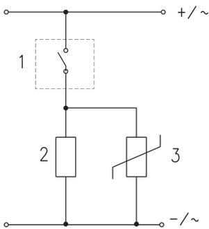
DC and AC applications: there is no protection on the Reed sensors on the inductive load, therefore it is advisable to use an electric circuit with protection against the voltage spikes. See picture above for a typical example.
