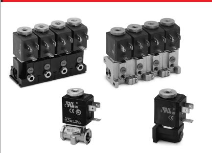
The solenoid can be easily and quickly replaced without interfering with the pressurised part of the valve. On the same mechanical part different types of solenoids can be interchanged. The choice of solenoids determines the performance of the solenoid valve in terms of consumption and pressure.
