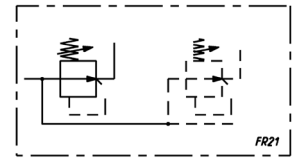
FR21 = Manifold regulator without relieving and without pressure gauge
